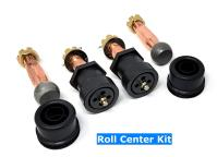
Extend Length Roll Center Pins are included separately and must be installed if you wish to use them. Keep the stock length pins in safe place in case you wish to return the car back to stock for resale purposes.
