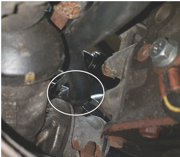
Fig 4 - factory reservoir hose to brass elbow
