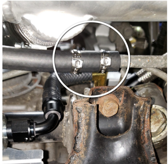
Fig 5 - 3/8" hose from new heat exchanger to factory hardline double pinch clamps
