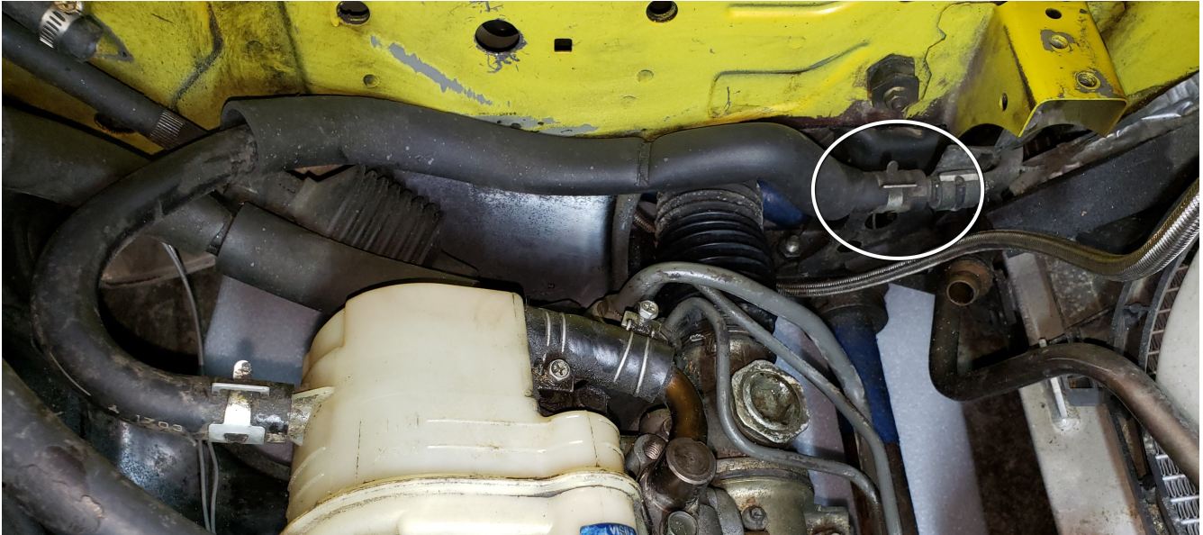
Fig 2: Remove Power Steering Hose From Factory PS Loop - To Be Connected To Brass Elbow (I)
