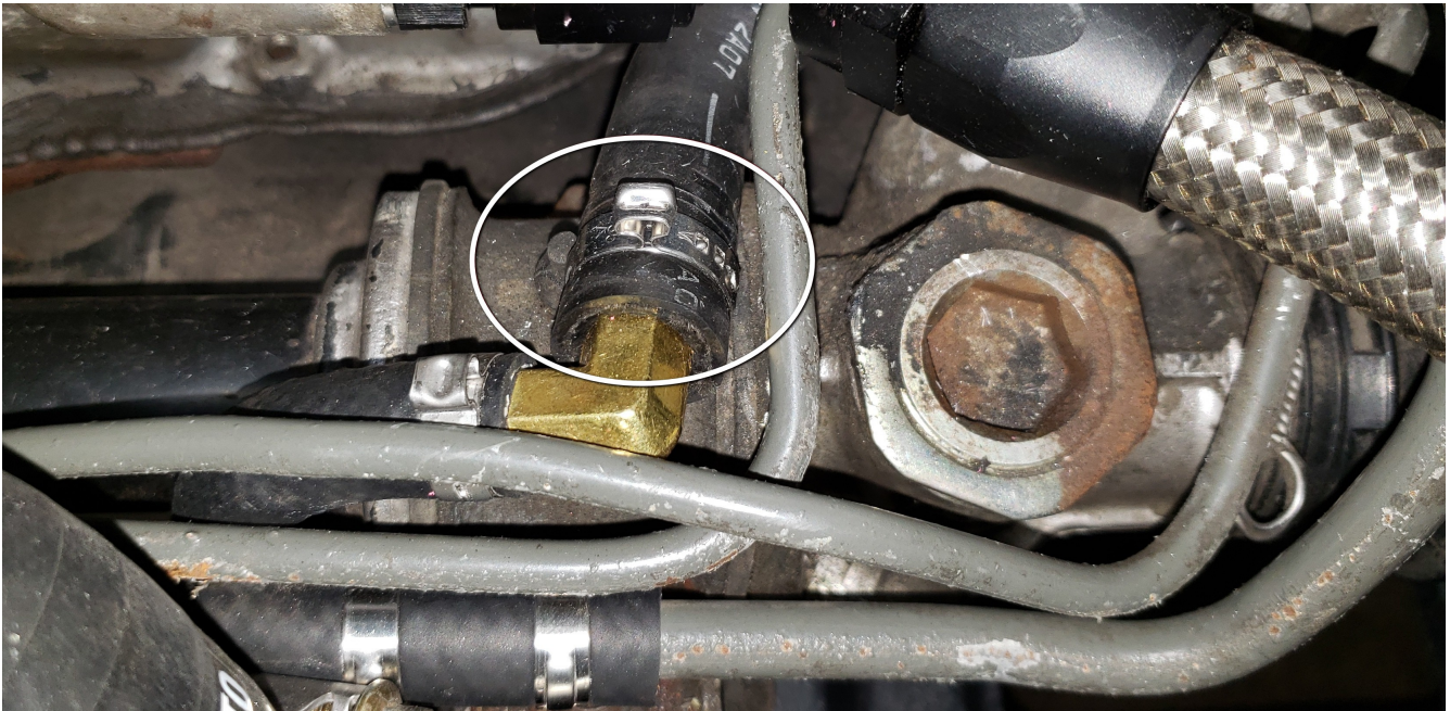
Fig 3: Power Steering Hose Connected To Reservoir
